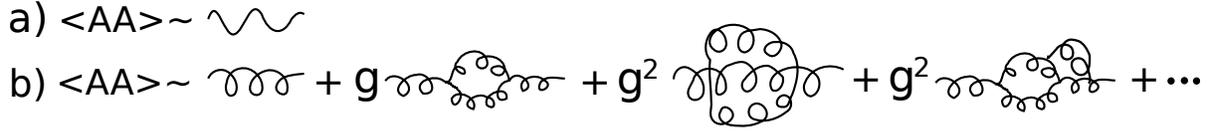
**Figure 3:** a) Photons have no self-interactions, so the tree-level propagator is exact. b) Gluons (and vector bosons) have 3-pt and 4-pt vertices, so there are loop contributions to the propagator.
